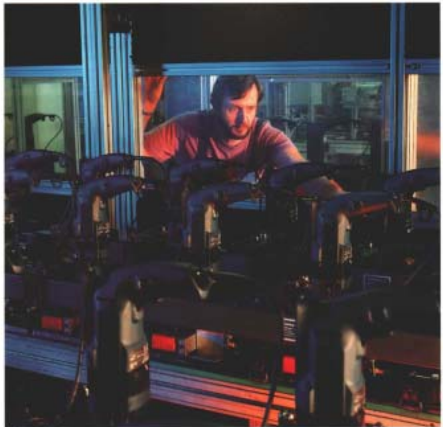
Endurance testing of hammer drills at our Swiss subsidiary Scintilla AG.
