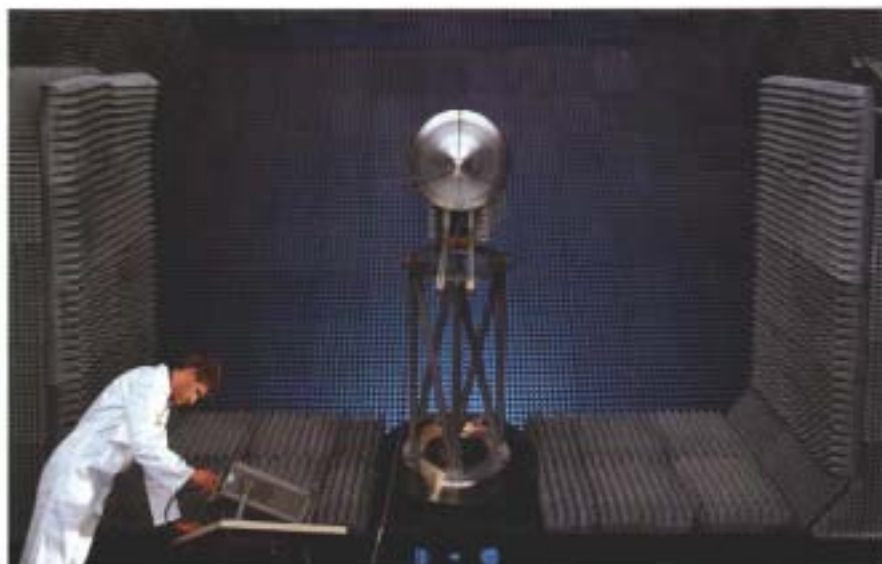
Testing the electrical properties of a satellite antenna inside an anechoic measuring chamber.
