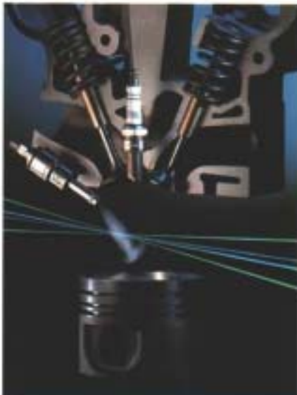
We are currently developing a number of components for fuel-efficient gasoline direct-injection. Our photo shows the analysis of air/fuel mixture formation using laser measurement technology.
