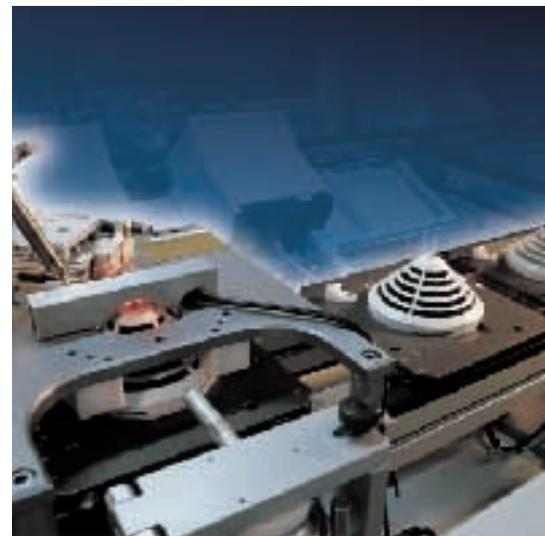
**Final examination for safety and reliability: Before our fire alarms leave the plant, we connect every single device to an alarm system and test all its functions.**
