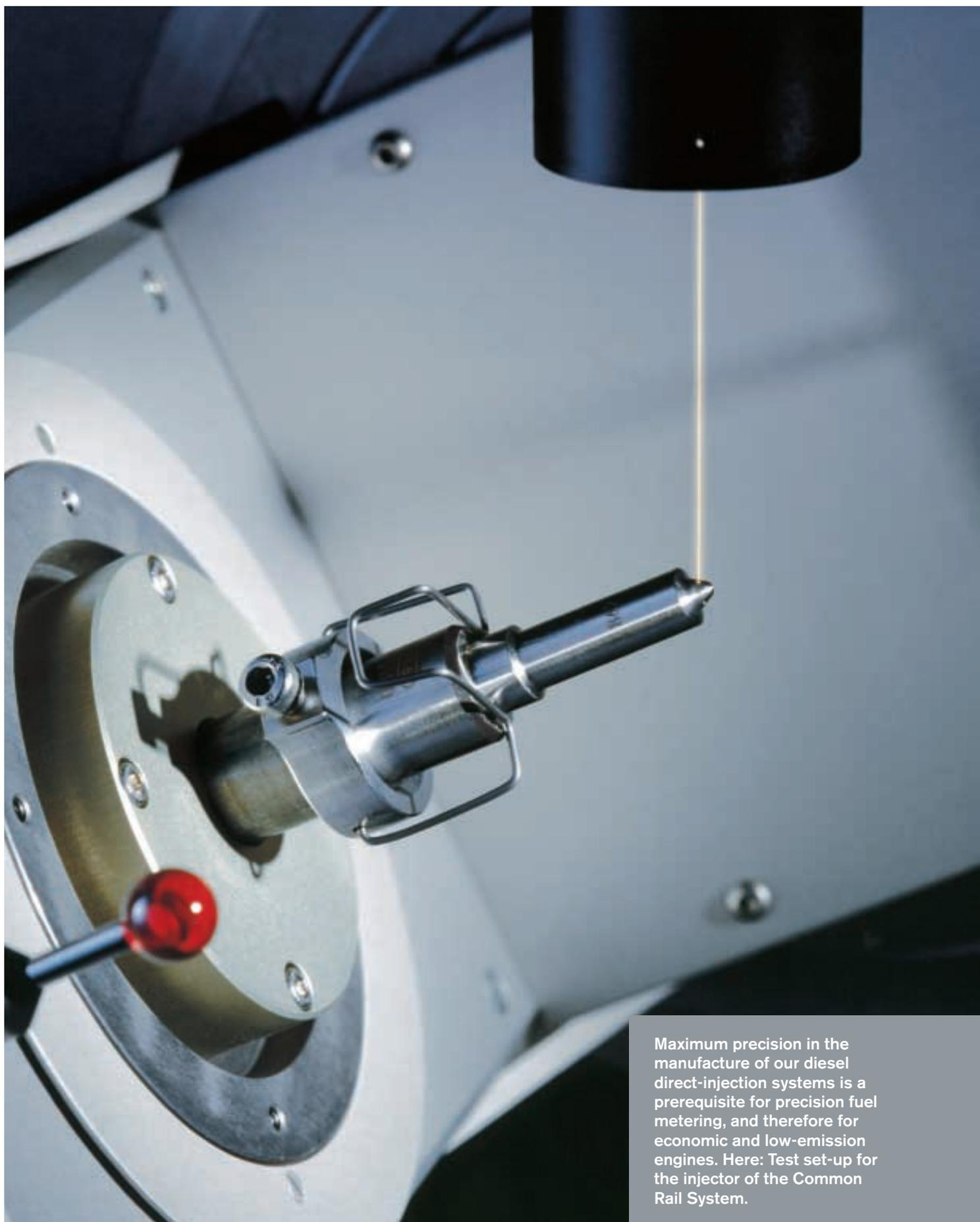
Maximum precision in the manufacture of our diesel direct-injection systems is a prerequisite for precision fuel metering, and therefore for economic and low-emission engines. Here: Test set-up for the injector of the Common Rail System.
