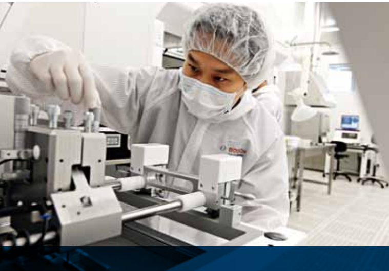
Research laboratory for the production of organic photovoltaic cells at our southeast Asian headquarters in Singapore. The photo shows a screen-printing machine being set up.
