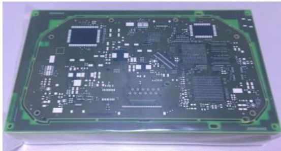
Figure 2: Stack of PCBs packed in a PE/PET foil.
