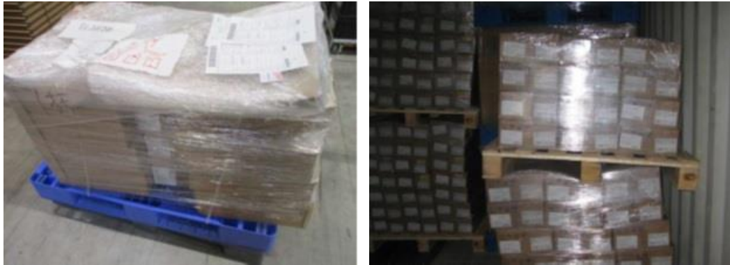
Figure 13: Damages due to wrong palletization and lack of exterior protection.
