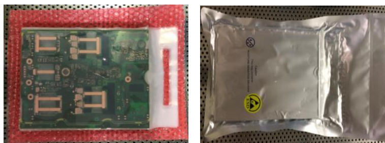
Figure 9: Solid stack of printed boards packed in a sealed moisture barrier bag (MBB).
