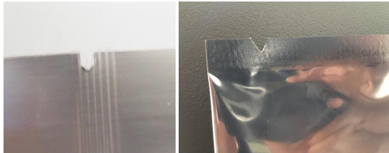
Figure 5: Example of “V” cut shape for opening the MBB bag.
