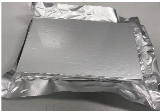
Figure 3: PE/PET foil packages packed in a sealed moisture barrier bag (MBB).
