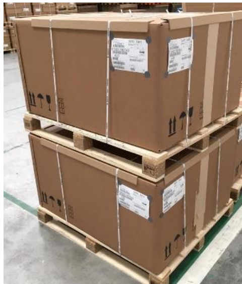
Figure 11: Dynamic stacking factor at least = 2 (1+1).
