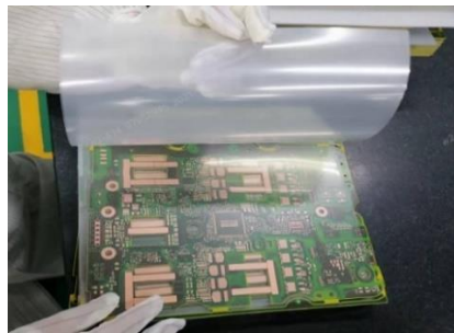
Figure 7: Separating layers between printed boards.
