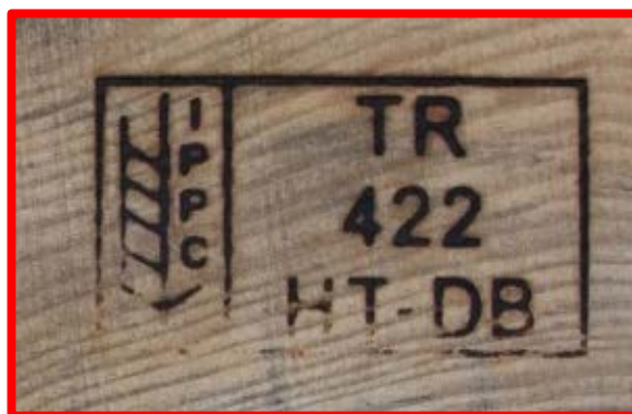
Figure 4: Not ok: frame incomplete, IPPC logo and HT marking not clearly readable
