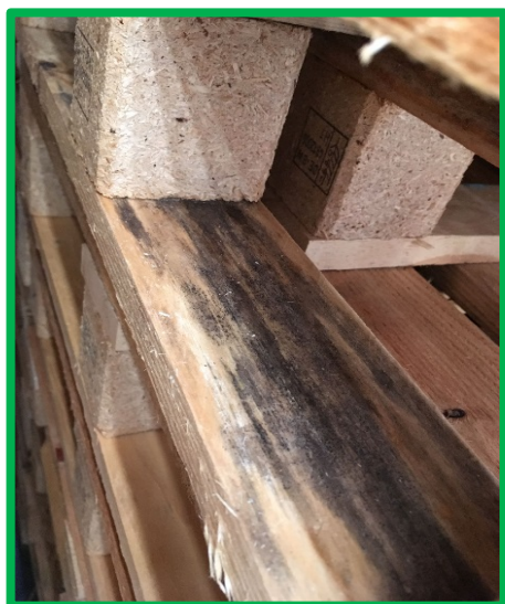
Figure 13: ok blue mould
