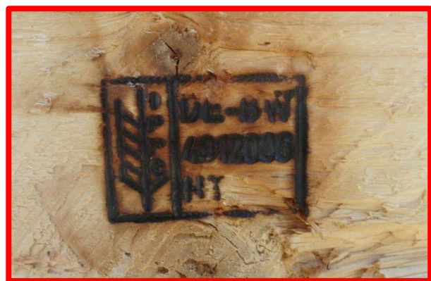
Figure 5: Not ok: planar surface burning, IPPC logo not clearly readable, Country code and supplier number not clearly readable
