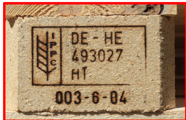
Figure 10: Not ok: frame incomplete, HT marking not clearly readable
