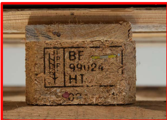
Figure 9: Not ok: Country code and supplier number not clearly readable, frame and IPPC logo incomplete
