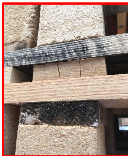
Figure 18: not ok, mould, sponge, dry rot
