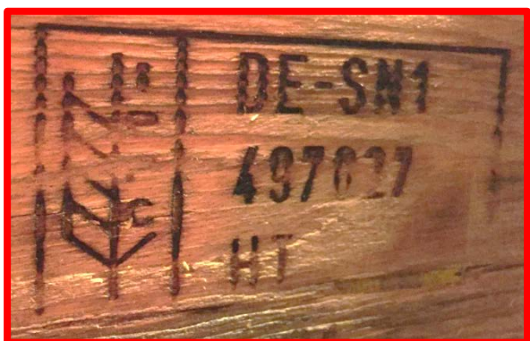
Figure 3: Not ok: Country code and supplier number not clearly readable, frame and IPPC logo incomplete
