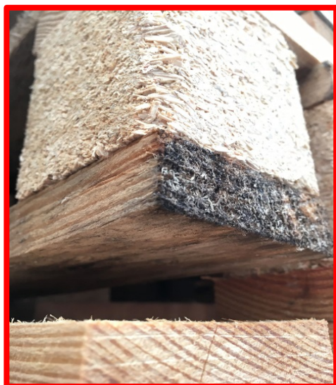
Figure 19: not ok, mould, sponge, dry rot
