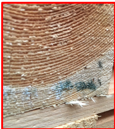
Figure 17: not ok, mould, sponge, dry rot
