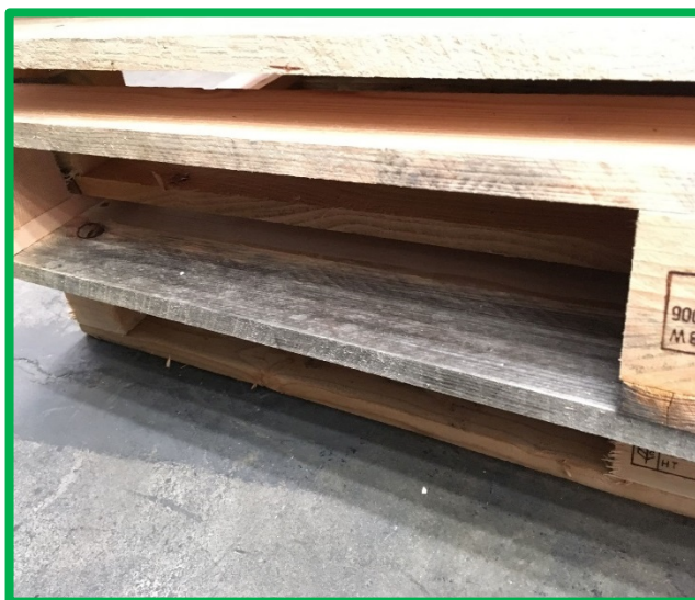
Figure 14: ok blue mould
