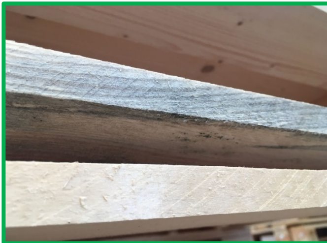
Figure 11: ok: blue mould
