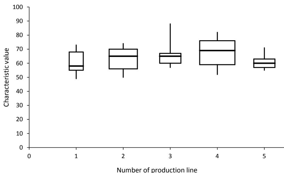
**Fig. 2.13:** Box plot of the characteristic values of injection valves which are manufactured on different production lines.
