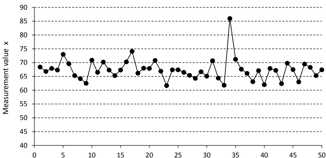
**Fig. 7:** Representation of the measurement values of the characteristic X in the form of a dot sequence
