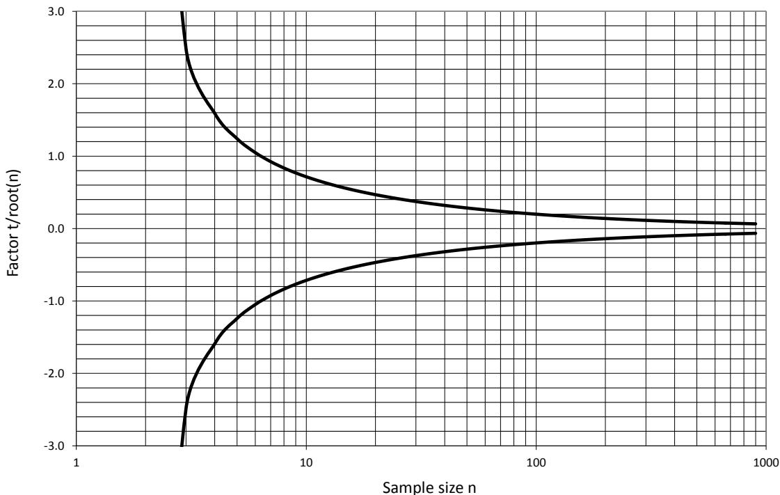
**Fig. 9:** The representation illustrates the dependence of the confidence interval of the mean  $\mu$  on the sample size  $n$ .
