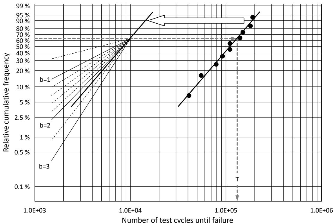
**Fig. 17:** Representation of the points in a Weibull plot: x-axis (= t-axis)
