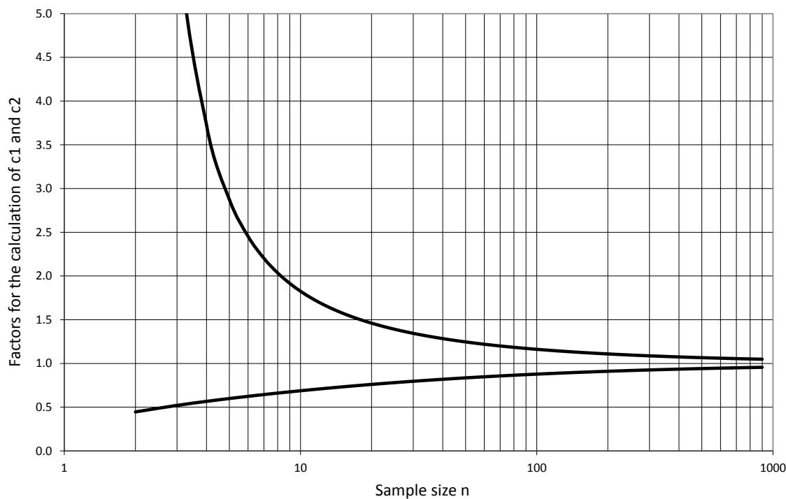
**Fig. 10:** The representation illustrates the dependency of the confidence interval of the standard deviation  $\sigma$  on the sample size  $n$ .
