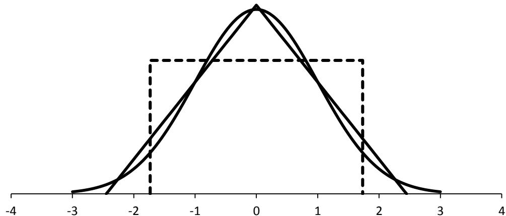
**Fig. 2:** Probability density functions of various distributions with the same standard deviation  $\sigma=1$  (see remark on the left side)
