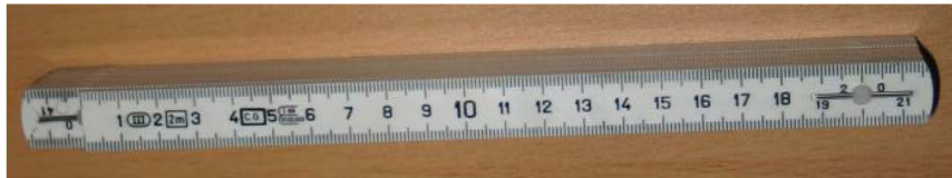
Figure 10: Commercially available folding ruler (accuracy class III, total length 2 m)
