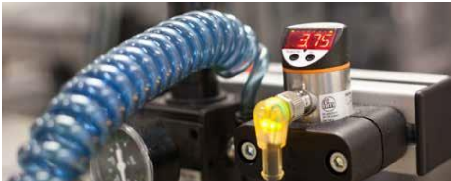
Figure 12: Digital display of a defined process parameter. The process parameter may only be changed by an authorized associate with a key.
