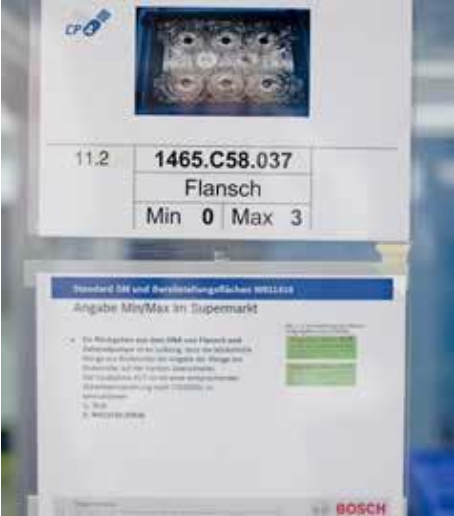
Figure 27 (left): Standardized marking of storage locations with specification of the minimum and maximum inventory Figure 28 (right): Storage of defective parts at a defined location
