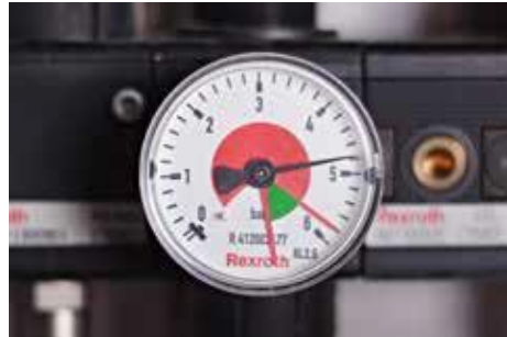
Figure 11: Colour coding of tolerance range; left: tolerance adhered to, right: process parameter outside tolerance range
