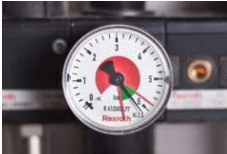
Figure 11: Colour coding of tolerance range; left: tolerance adhered to, right: process parameter outside tolerance range
