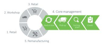
The used parts from vehicles are removed from the market, identified, and sorted in a structured manner. Provided that they meet technical requirements, they are then sent to production and remanufacturing. In order to ensure a seamless return process, in 2016 Bosch founded the Circular Economy Solutions subsidiary. Under the CoremanNet brand name, the company removed 2.5 million parts from the market in 2016.
